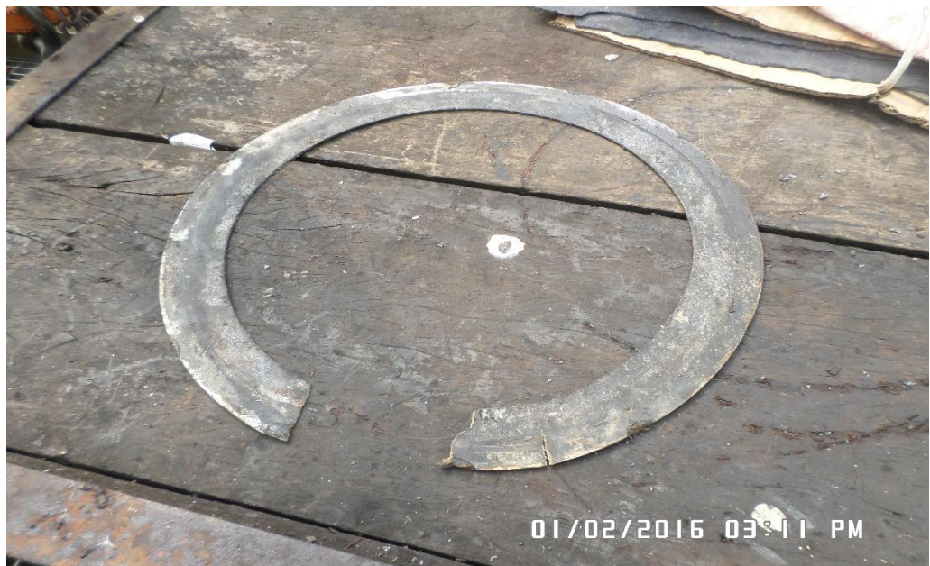
Figure 2.2. Failed orifice (Seal)
